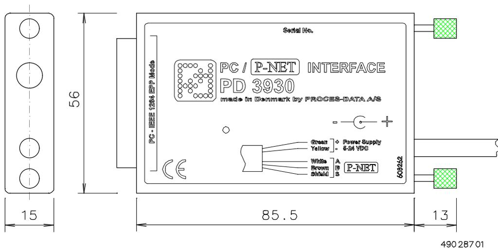
PD 3930 is approved in compliance with the EMC-directive no 89/336/EEC. Test limits are determined by the generic standards EN 50081-1 for emission and EN 50082-2 for immunity. PD 3930 is approved in compliance with the IEC 68-2-6 Test Fc standard for vibration.
